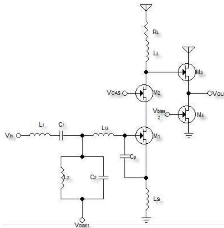
Figure 15: Source degenerated common source amplifier, [Bevi 04]
