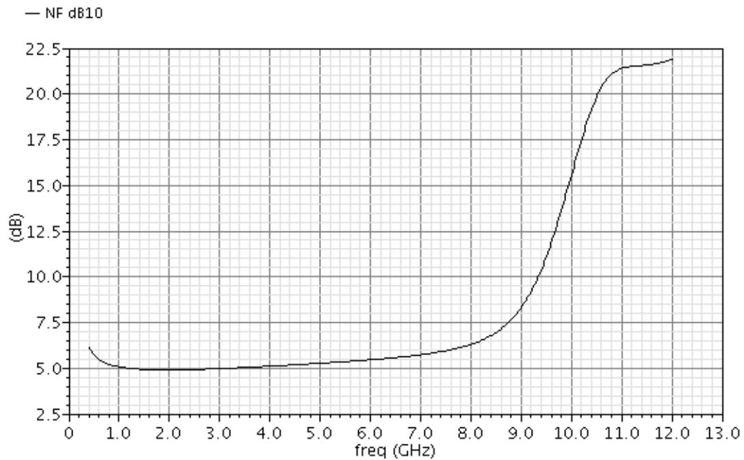
Figure 37: Post-layout simulated NF of LNA 4
