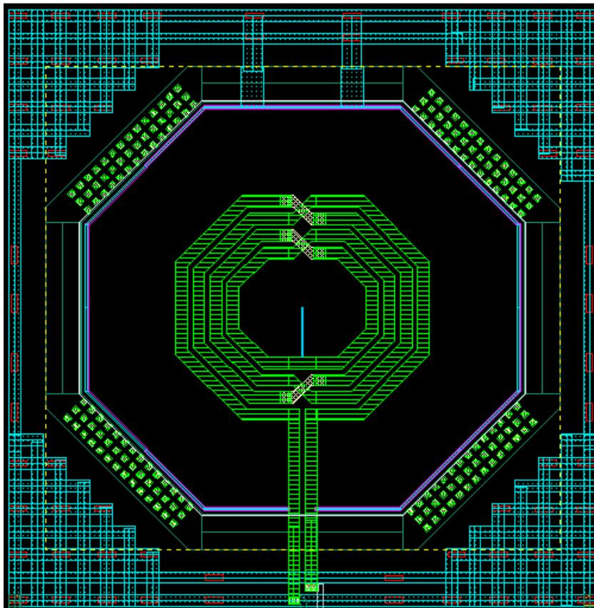
Figure 47: Inductor on chip with metal grid
