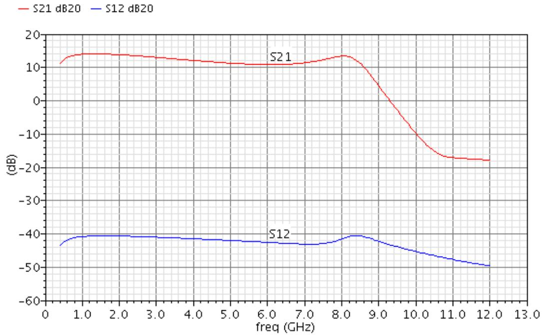
Figure 36: Post-layout simulated  $S_{21}$  and  $S_{12}$  of LNA 4
