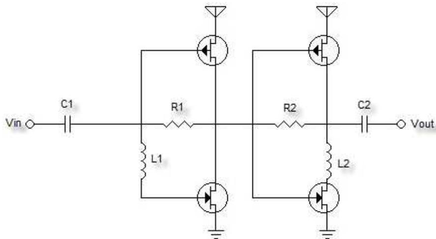
Figure 24: Schematic LNA 2
