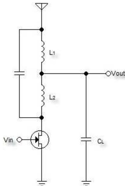
Figure 8: T-coiled enhanced common source amplifier
