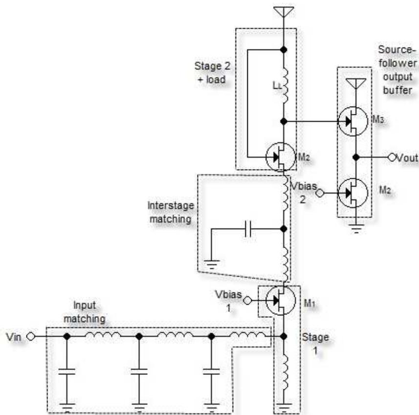
Figure 16: Common gate amplifier with interstage matching network [Stan 05]
