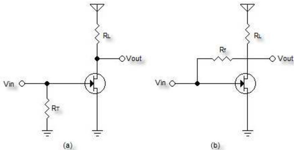
Figure 4: Generic wideband impedance matching solutions. A: Resistor terminated common-source. B: Shunt feedback common-source.
