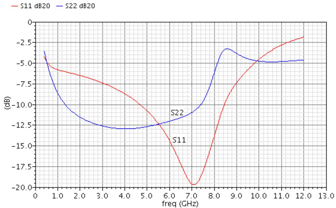
Figure 35: Post-layout simulated  $S_{11}$  and  $S_{22}$  of LNA 4
