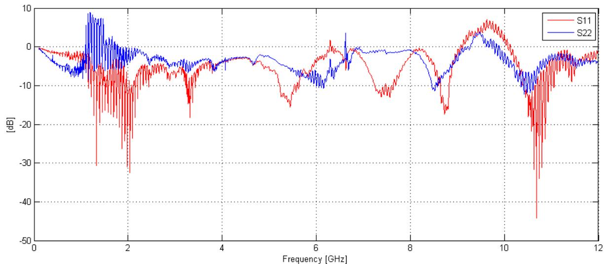
Figure 54: Measured  $S_{11}$  and  $S_{22}$  of LNA 2
