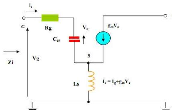
Figure 10: Small signal equivalent of a source degenerated transistor<sup>1</sup>
