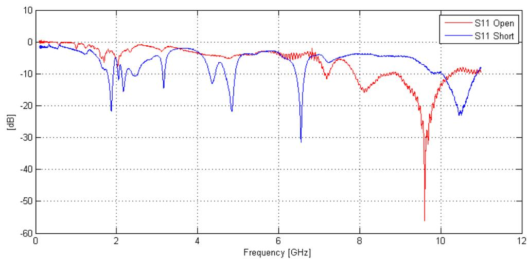
**Figure 60: Measured  $S_{11}$  of shorted and open bond wire test benches implemented on test chip**
