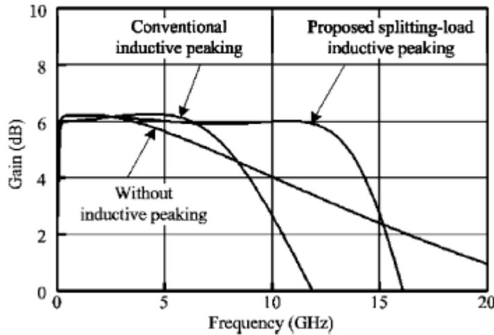
Figure 19: Simulated gain performance of single state inverters. From [Chao 08], copyright © 2008 IEEE
