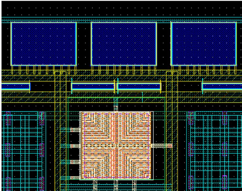
Figure 44: Decoupling included in the LNA layouts
