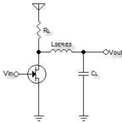
Figure 6: Series peaked common source amplifier
