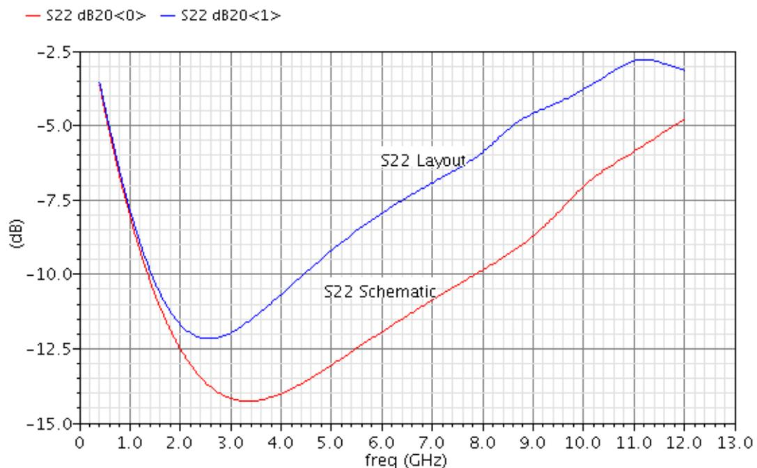
Figure 29: Post-layout versus schematic  $S_{22}$  simulations of LNA 3
