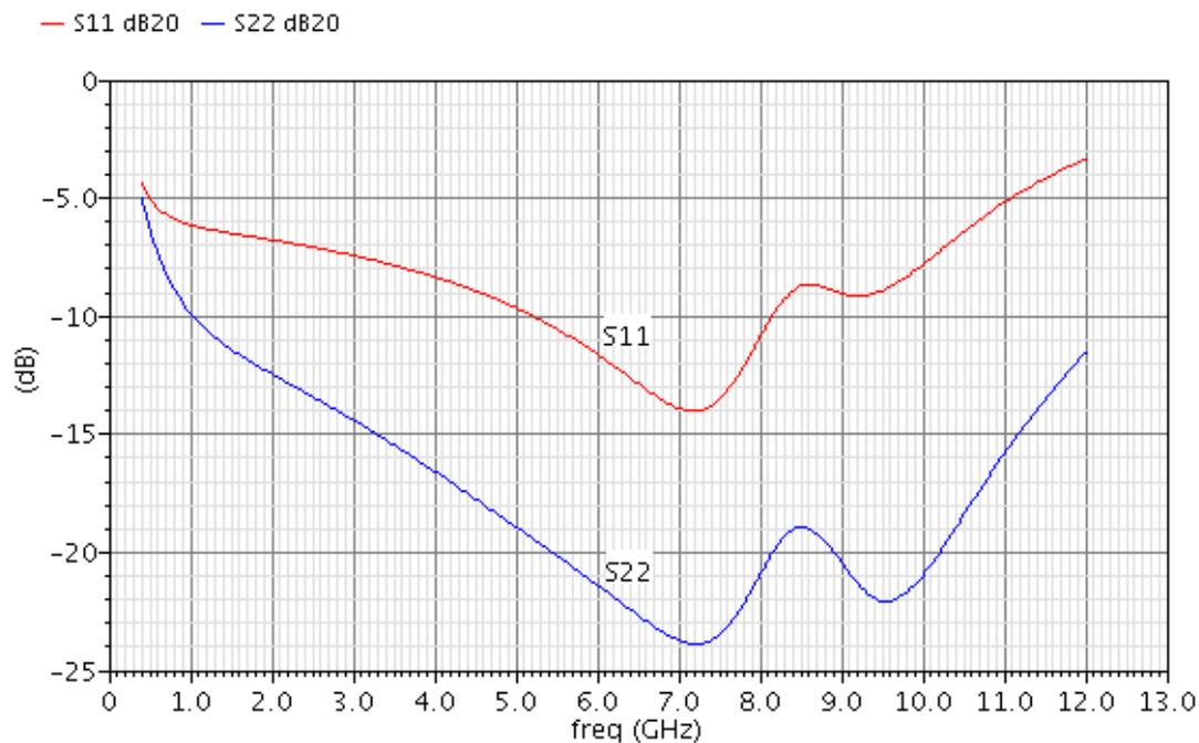
Figure 21: Layout simulated,  $S_{11}$  and  $S_{22}$ , of LNA 1
