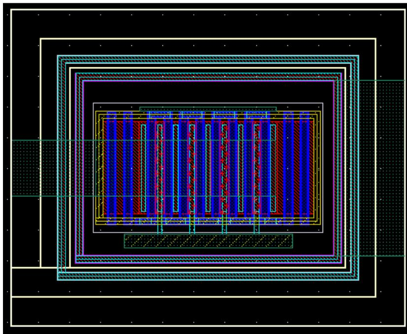
Figure 45: Layout of RF NMOS provided by the design kit
