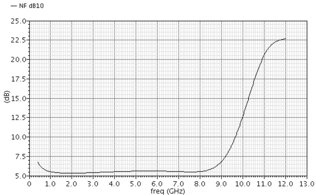
**Figure 23: Layout simulated NF of LNA 1**
