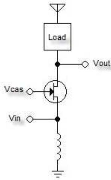
Figure 11: Common gate amplifier
