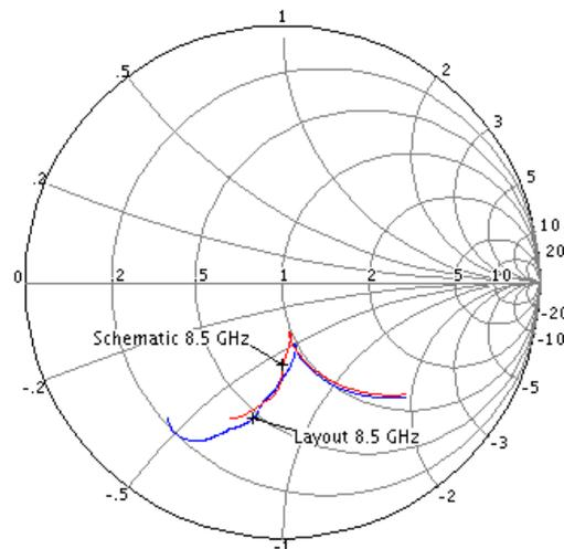
**Figure 30: Post-layout versus schematic  $S_{22}$  simulations of LNA 3**
