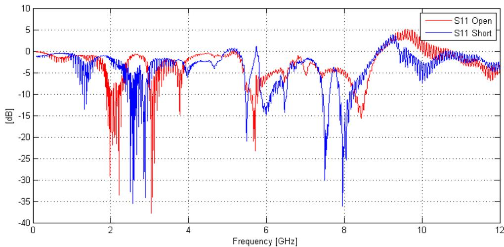
**Figure 58: Measured  $S_{11}$  of shorted and open bond wire test benches implemented on master chip**
