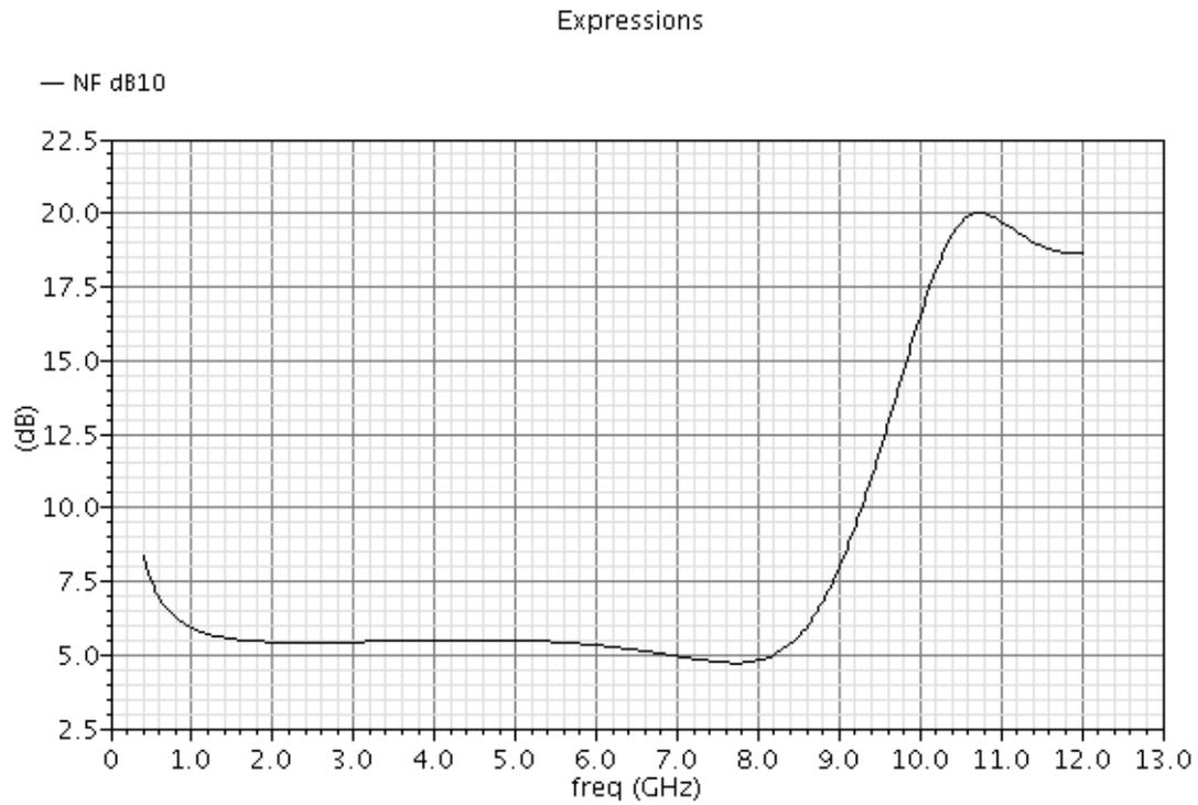
**Figure 33: Post-layout simulated NF of LNA 3**
