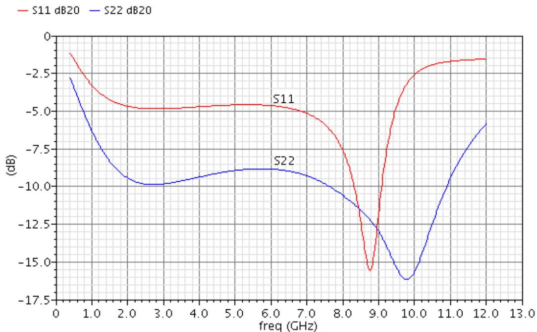
Figure 25: Post-layout simulated  $S_{11}$  and  $S_{22}$ , of LNA 2
