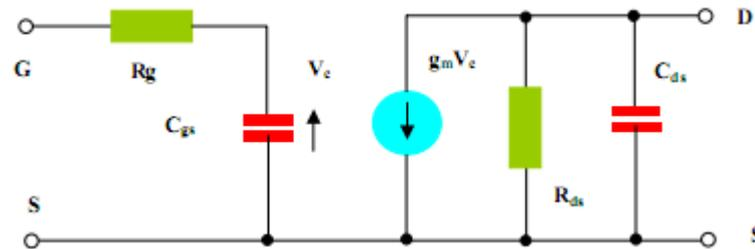
Figure 12: Small signal equivalent<sup>2</sup>
