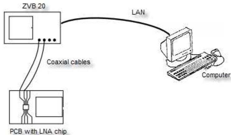
Figure 51: Measurement setup, inspired by [Dahl 09]
