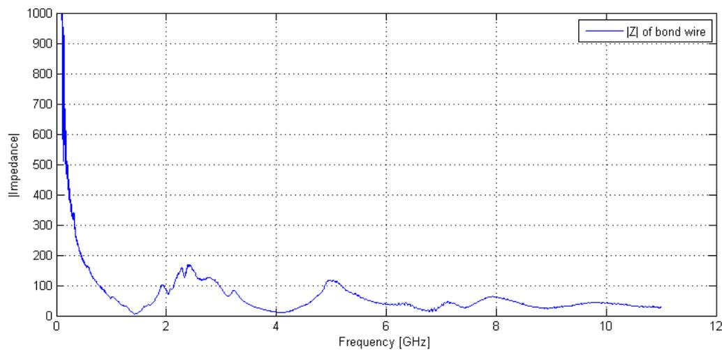
**Figure 61: Calculated absolute value of impedance in bond wire of test chip using W. C. Johnson Formula**
