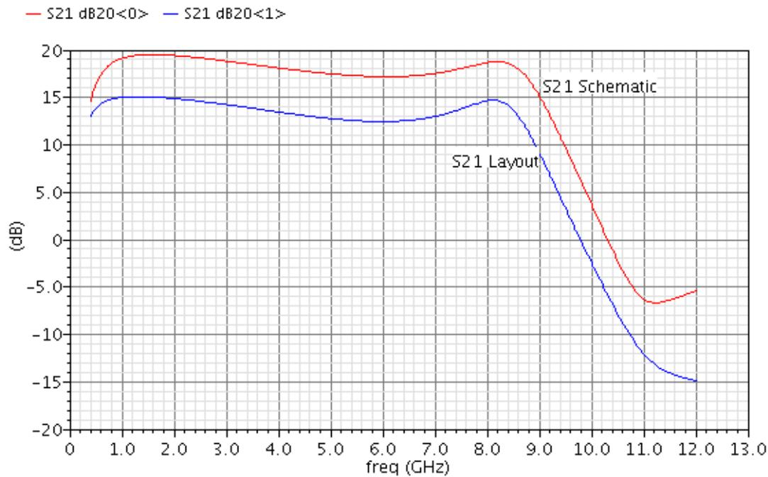
Figure 40: Simulated power gain,  $S_{21}$ , of LNA 1 in schematic and post-layout
