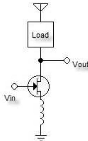
Figure 9: Common source amplifier
