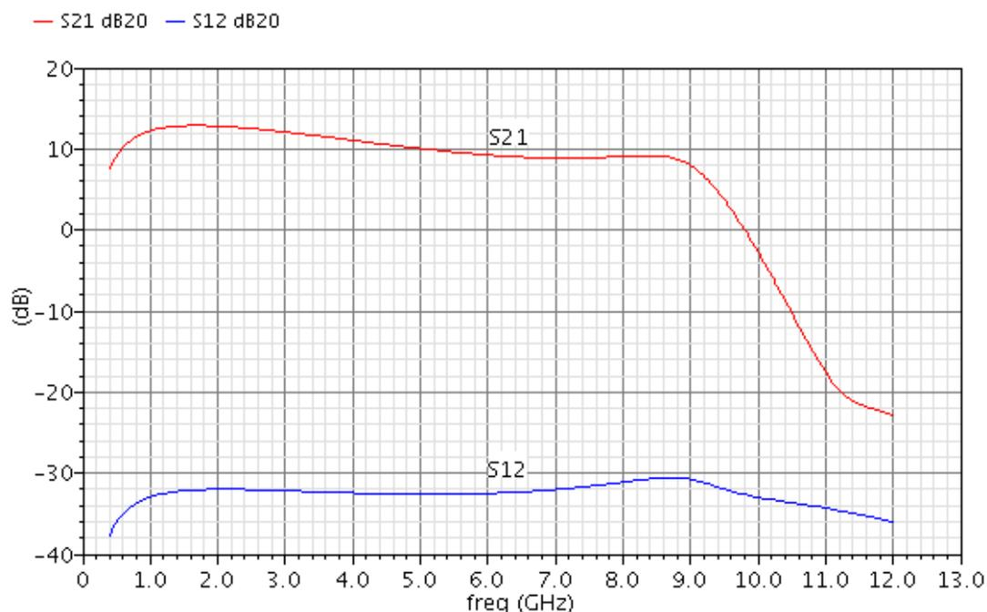
Figure 26: Post-layout simulated  $S_{21}$  and  $S_{12}$ , of LNA 2
