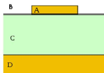
Figure 48: Cross-section of a PCB with microstrip line<sup>3</sup>
