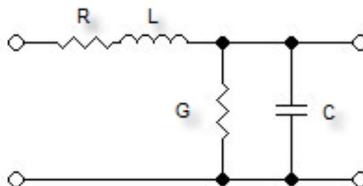
Figure 1: Unit transmission line element
