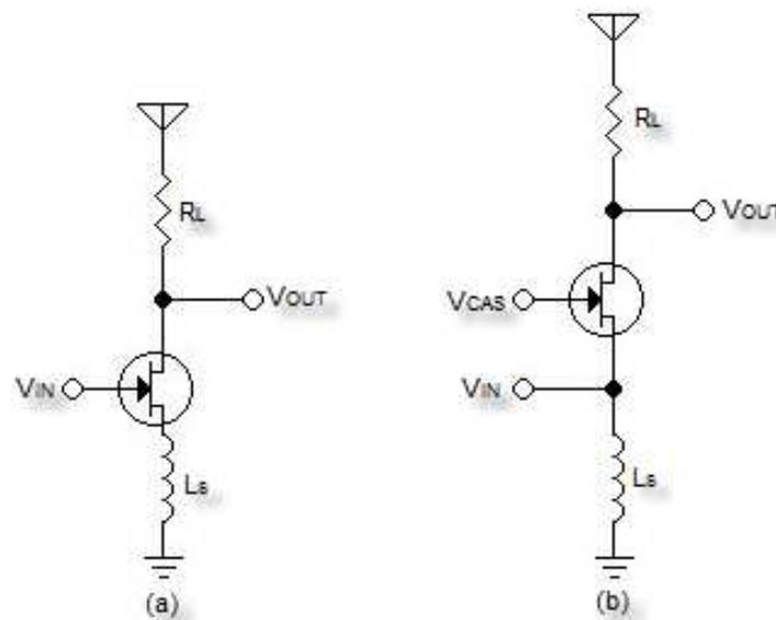
**Figure 5: High frequency, wide band matching approaches. A: inductor degenerated common source. B: Common-gate**
