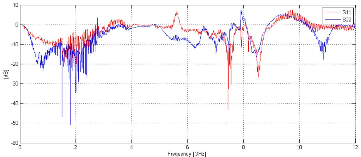
**Figure 52: Measured  $S_{11}$  and  $S_{22}$  of LNA 1**
