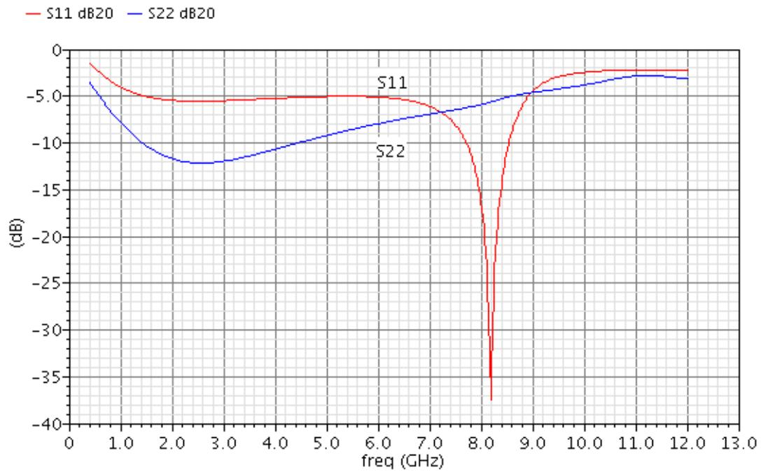
**Figure 31: Post-layout simulated  $S_{11}$  and  $S_{22}$ , of LNA 3**
