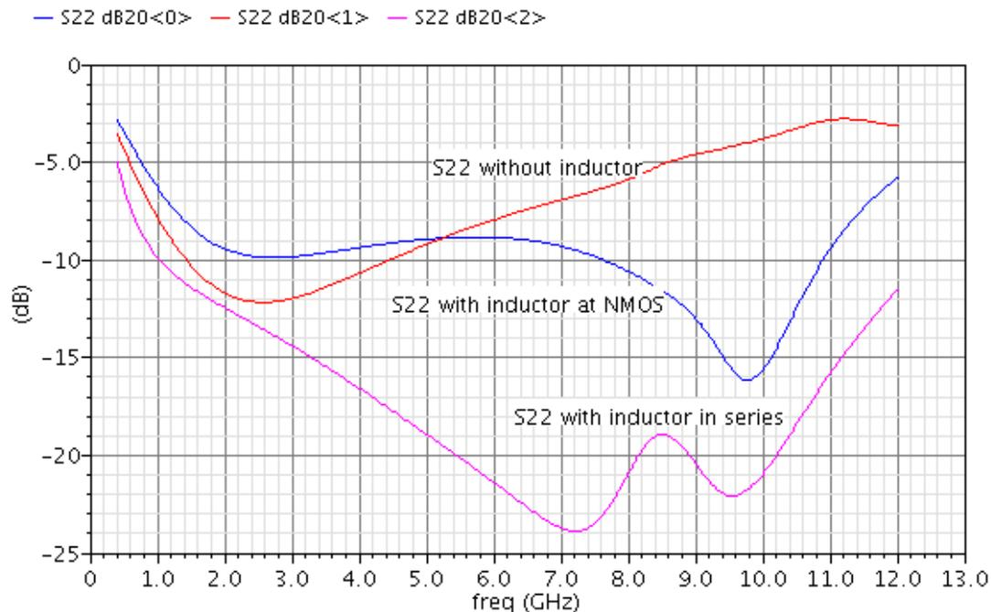
Figure 39: Post-layout simulated  $S_{22}$ , no inductor versus inductor at NMOS and inductor in series
