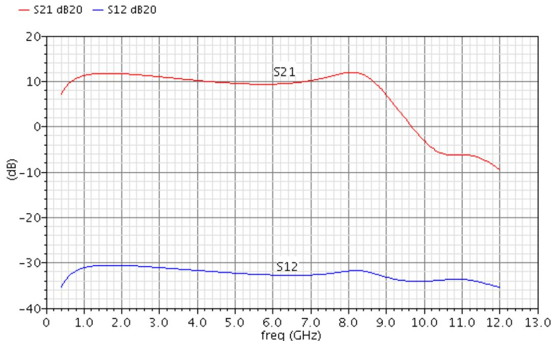
Figure 32: Post-layout simulated  $S_{21}$  and  $S_{12}$ , of LNA 3
