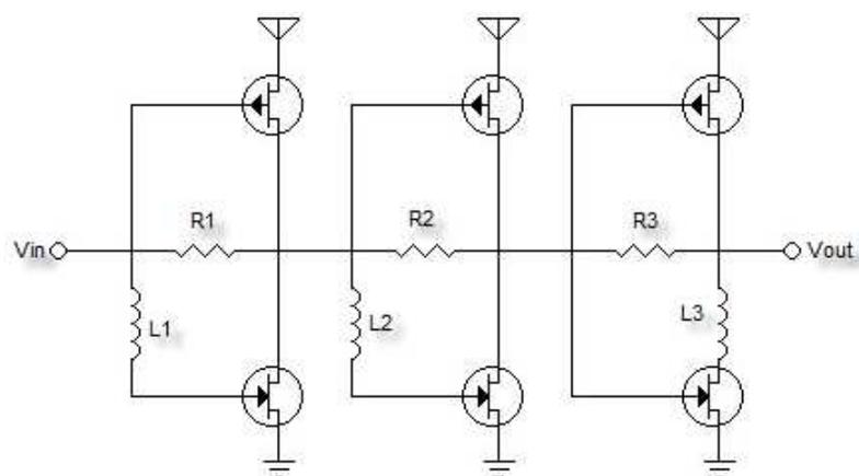
**Figure 18: Inverter based amplifier using splitting-load inductive peaking technique [Chao 08]**
