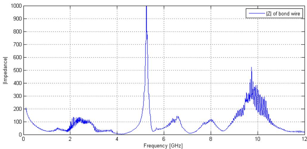
**Figure 59: Calculated absolute value of impedance in bond wire of master chip using W. C. Johnson Formula**
