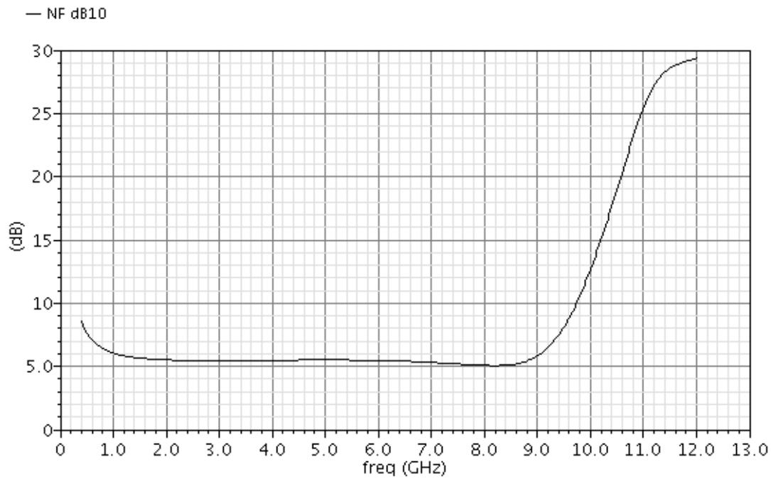
Figure 27: Post-layout simulated NF of LNA 2
