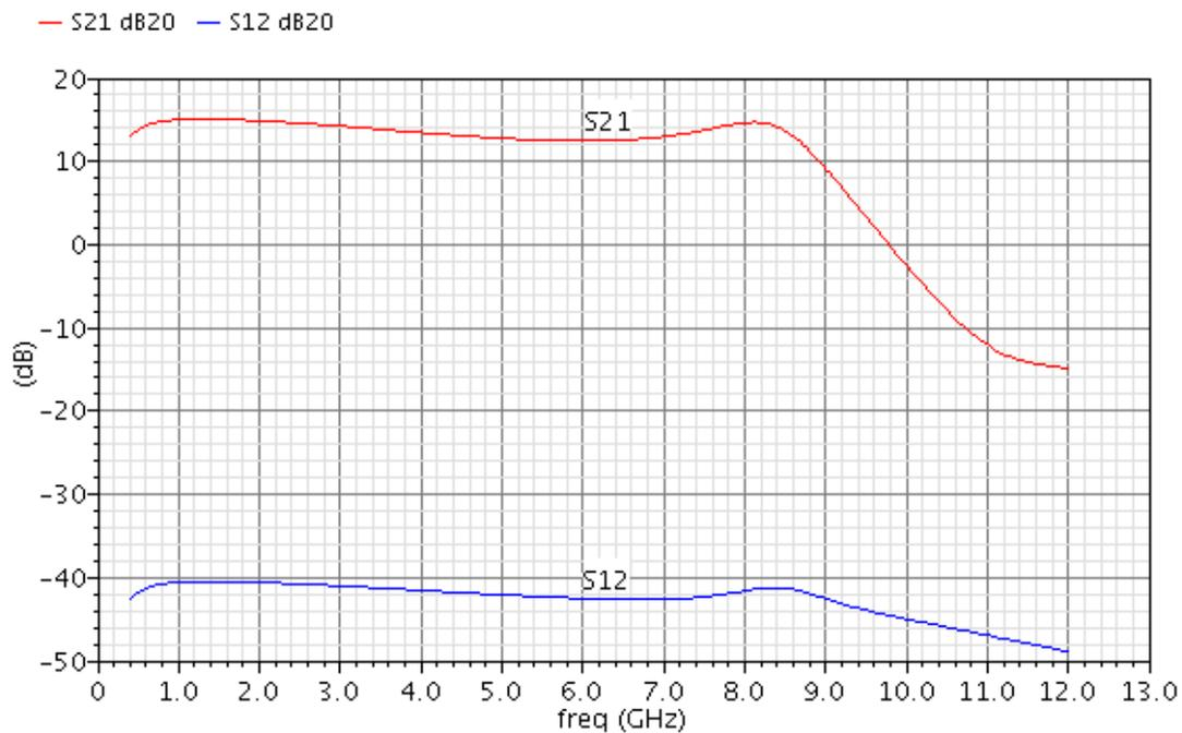
Figure 22: Layout simulated  $S_{21}$  and  $S_{12}$ , of LNA 1
