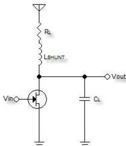
Figure 7: Shunt-peaked common source amplifier
