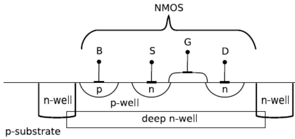
Figure 46: Cross section deep n-well NMOS, from [Dahl 09]
