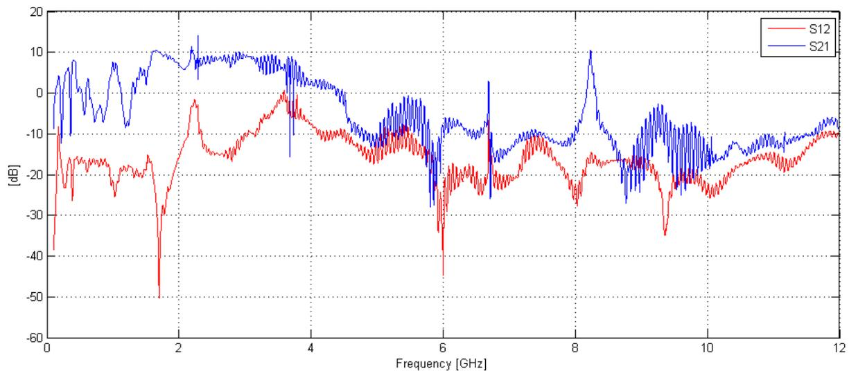
**Figure 57: Measured  $S_{21}$  and  $S_{12}$  of LNA 4**
