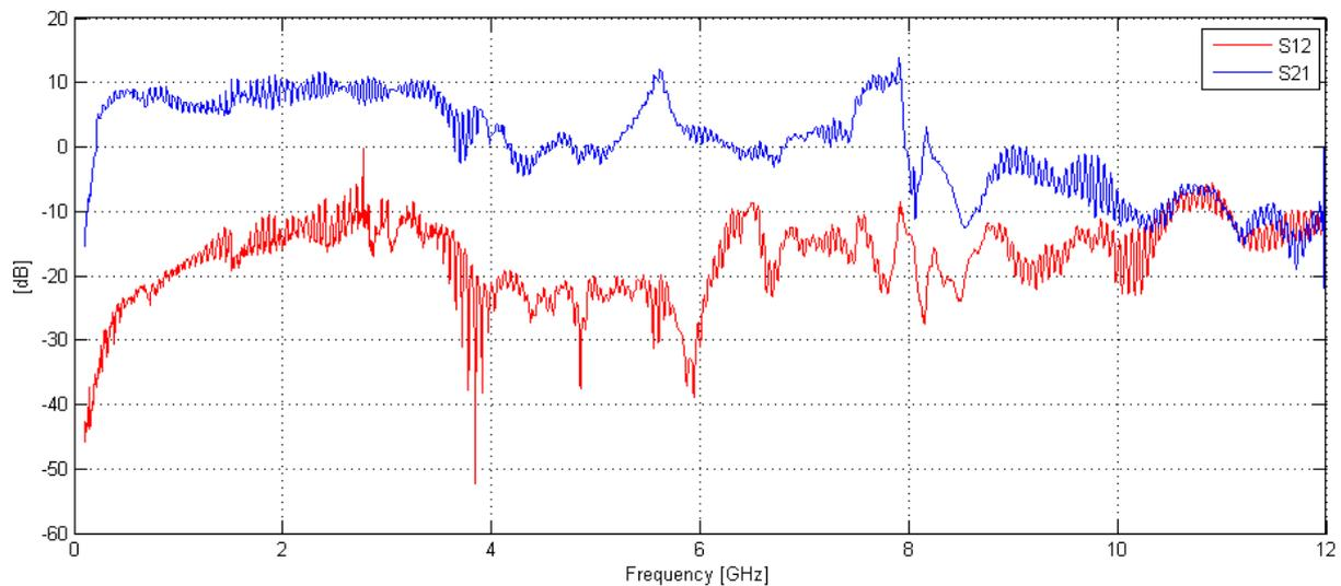
**Figure 53: Measured  $S_{21}$  and  $S_{12}$  of LNA1**
