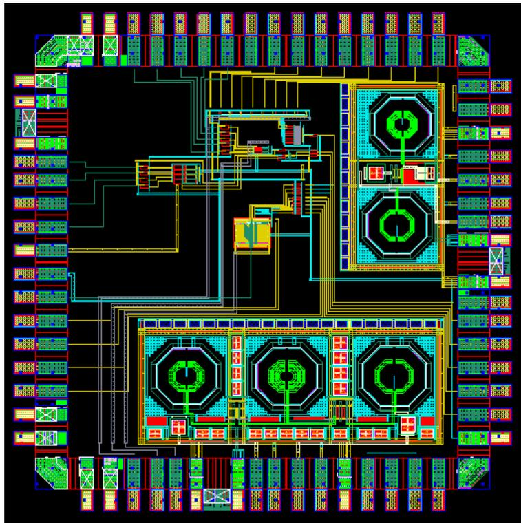
Figure 41: Pad frame of master chip
