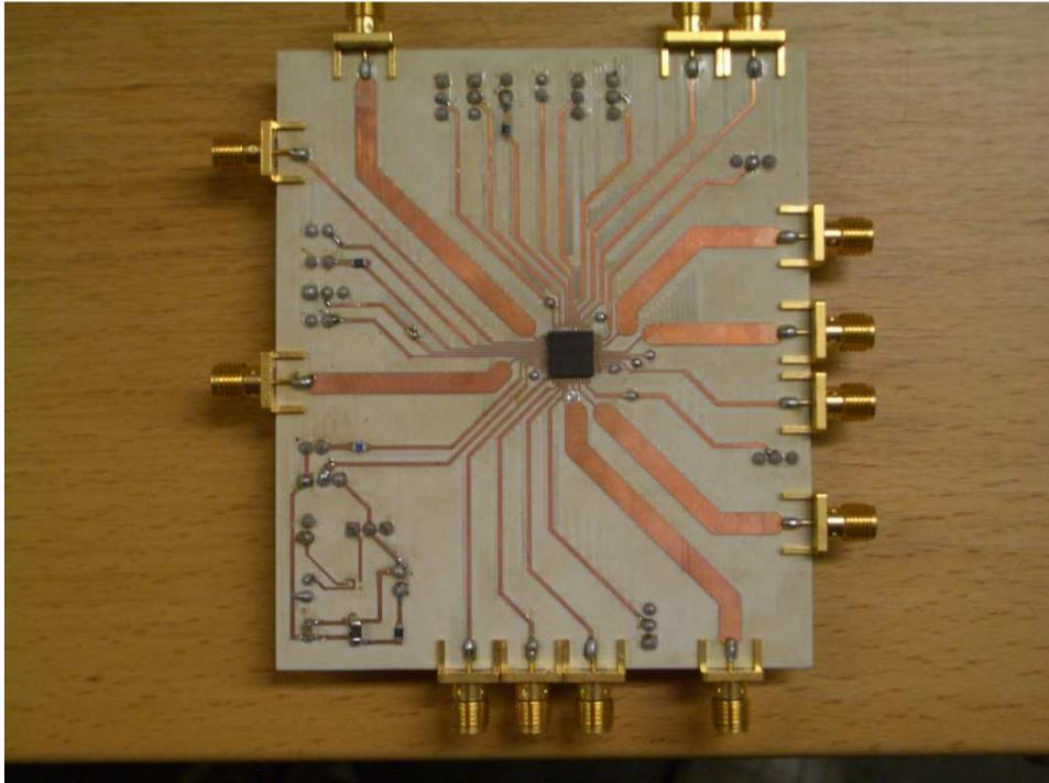
Figure 50: PCB of test chip
