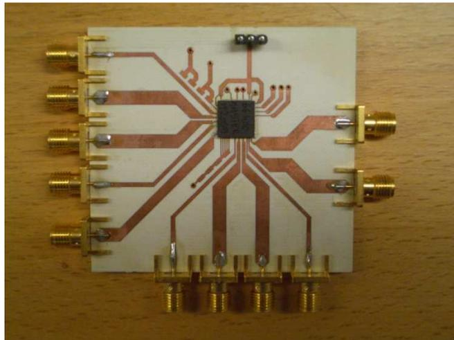
**Figure 49: PCB of master chip**
