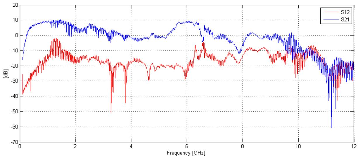
**Figure 55: Measured  $S_{21}$  and  $S_{12}$  of LNA 2**
