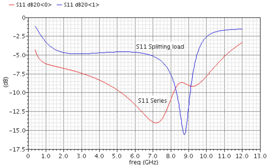
Figure 38: Post-layout simulated  $S_{11}$ , series match versus splitting load technique
