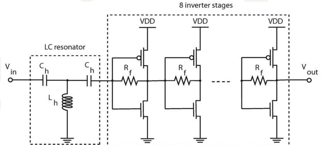
A resonant peak at the amplifier corner frequency can 'pull up' the gain, thus extending the bandwidth significantly.
