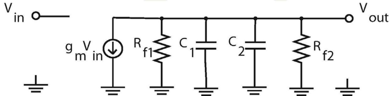
Considering the inter-stage small signal model, the transfer function can be expressed as [7]:
