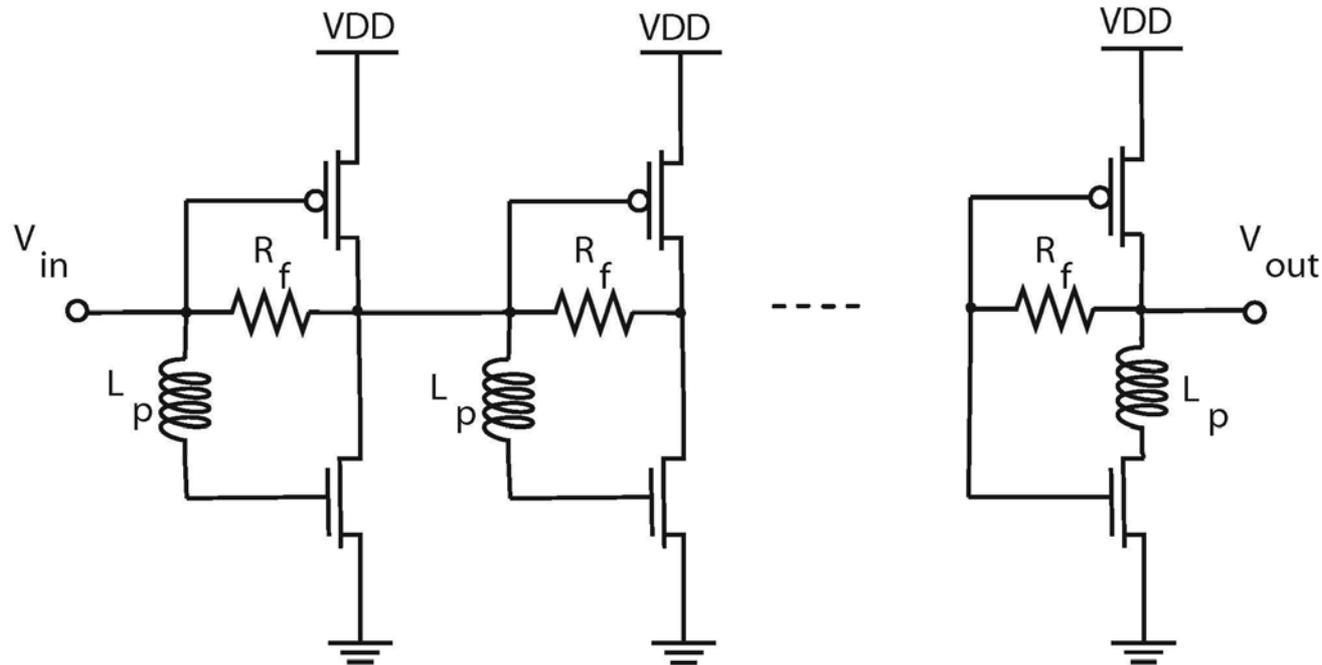
By locating a peaking inductor at the gate of nMOS of each inverter stage, the -3dB roll-off frequency can be boosted to higher frequencies.
