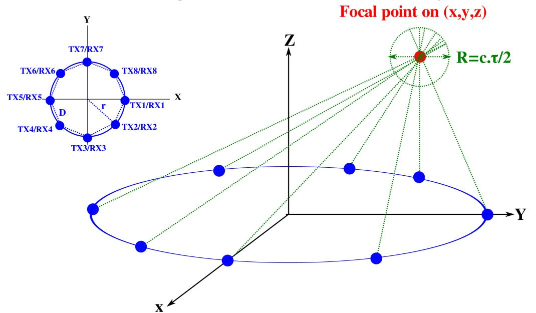
• All data from 8 receivers are processed in the software to construct a 3D image.
